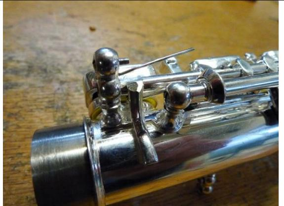
High C (thumb key on normal flute). The main axis has 3 layers; C key is on middle layer.
