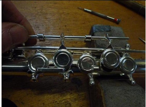
This is the bB rocker. Has its own spring. The long arm goes under the bB plastic roller. The long arm moves to the flute body when the spring is on. Some of them have a small piece of red plastic glued on (epoxy). If gone, replace with some 2mm material.
