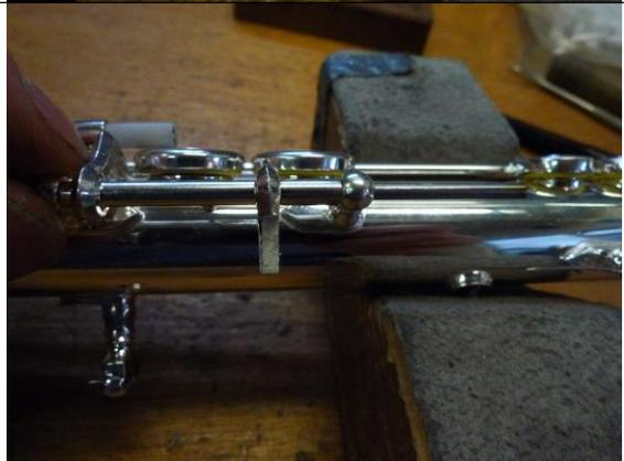
Then the lower thumb key. This operates the high #C key.
